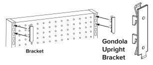
Insert Bracket hooks into top gondola slots, then push down to secure Bracket.
