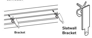
Insert Bracket up into slatwall opening. Rotate Bracket down to secure in place.
