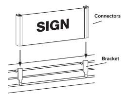
NOTE: The channel on the back of the Connector slides over the Bracket. Slide Connectors down onto Brackets.
