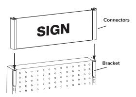
NOTE: The channel on the back of the Connector slides over the Bracket. Slide Connectors down onto Brackets.
